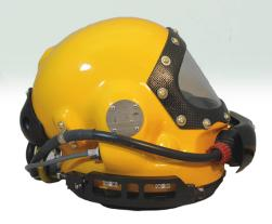
The DSL A-2air IV airhat has two one-way-breathing-circuits which are separated from each other and one separate and manually adjustable freeflow and defog system to keep the screen clean. The airdistribution block is compact and fixed at the worker's belt or harness.
