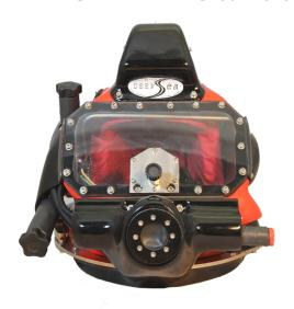
The DSL B-2 Caribe diving helmet is a surface demand life support system. Equipped with a standard SCUBAPRO A700 demandvalve, the demand valve adjustment allows an optimal breathing comfort. It has a neutral buoyancy for an optimized comfort underwater and a quarter-turn valve ensures a rapid bailout opening in case of emergency.
