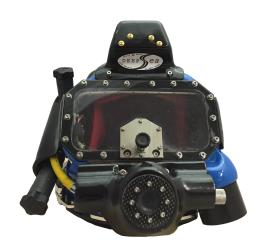
The removable ballast is designed to fit all DSL B-2 Nuclear and DSL B-2 Caribe diving helmets. It is built to be removed and put back on the helmet in less than 15 seconds. This system increases the working comfort to the diver when they have to wait on surface and cannot remove the helmet.
