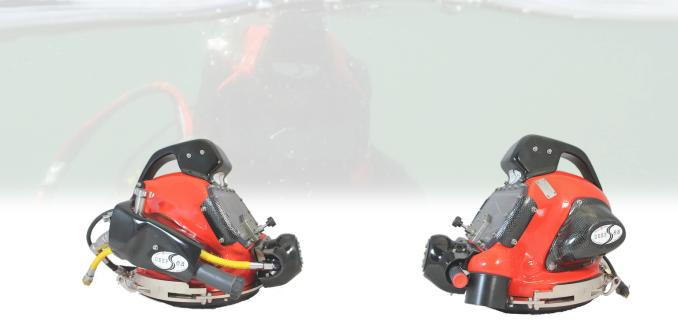
The DSL B-2 Nuclear is mounted with a double spring loaded overpressure valve to ensure the divers security in polluted media. This system ensures a constant overpressure of 5mB inside the helmet and avoids the flow-back of any poisoned particles.
